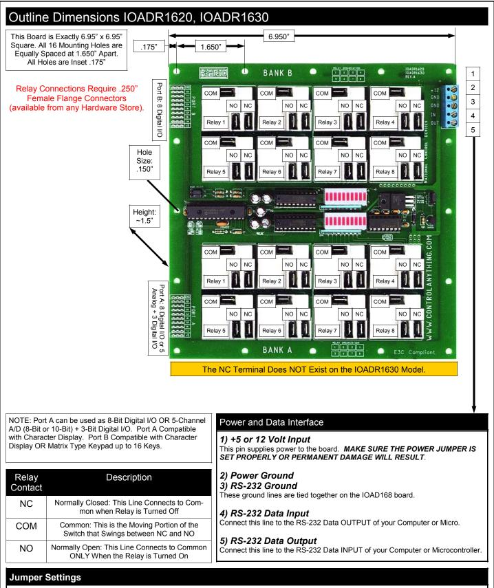
Set Jumpers to Configure Baud Rate. Settings are Printed on Circuit Board. Supported Baud Rates: 2400, 9600, 19.2K, or 38.4K Baud. Serial Configuration is 8 Data Bits, 1 Stop Bit, No Parity. This Controller Reads Jumper Settings when Power is First Applied to the Board ONLY.
