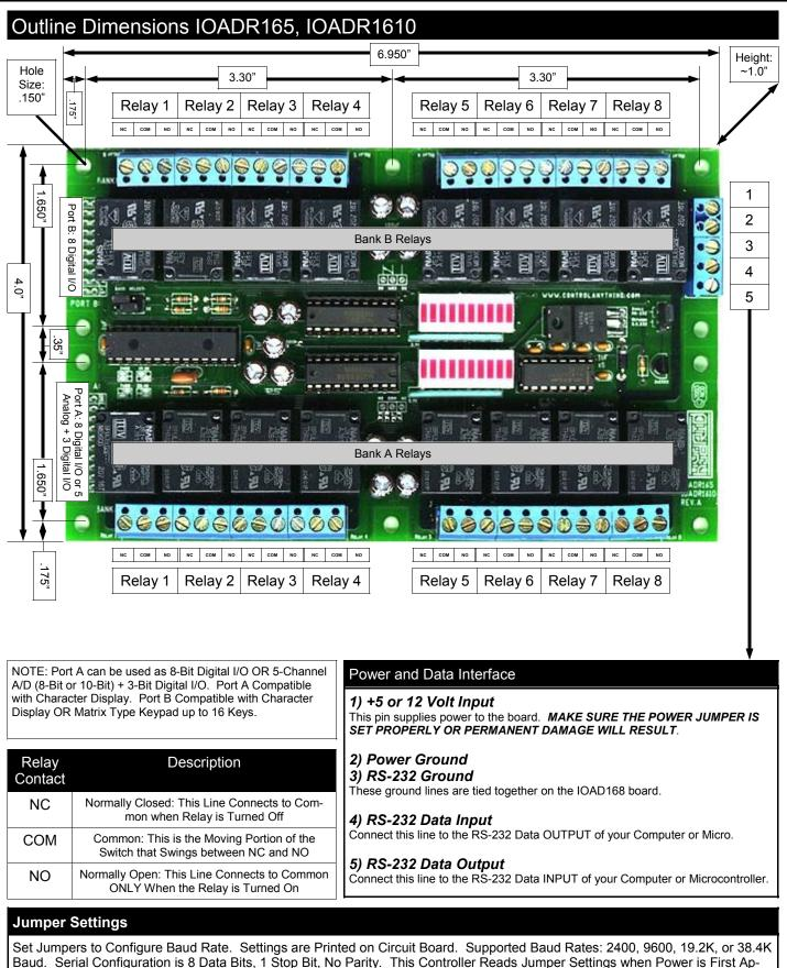
Baud. Serial Configuration is 8 Data Bits, 1 Stop Bit, No Parity. This Controller Reads Jumper Settings when Po plied to the Board ONLY.
