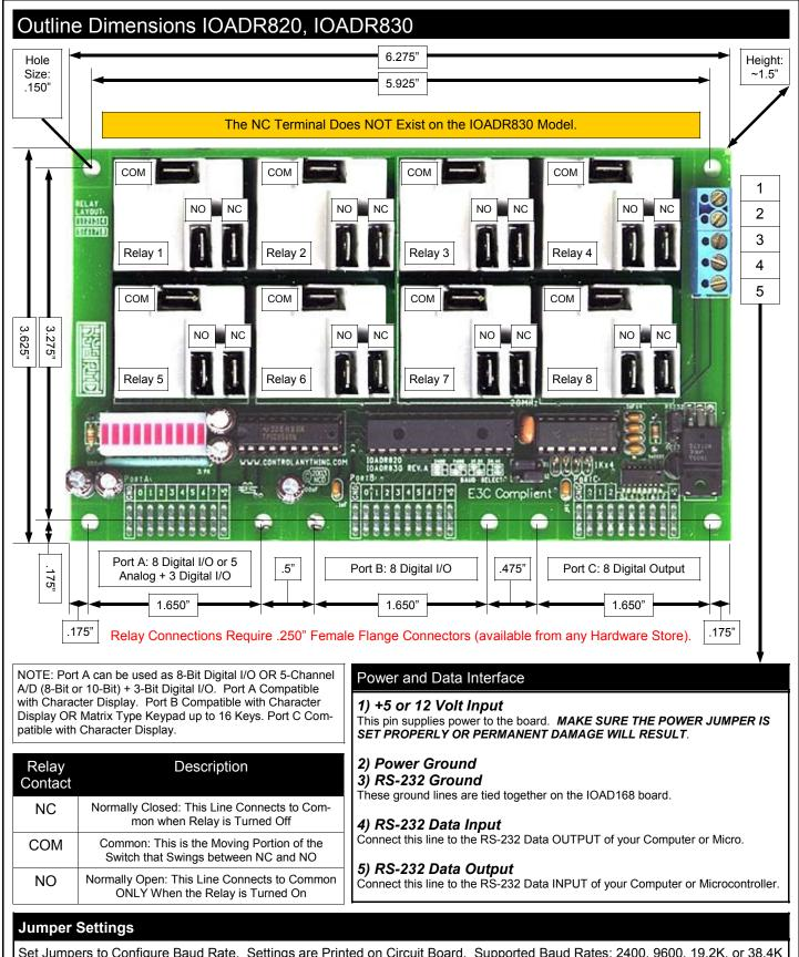
Set Jumpers to Configure Baud Rate. Settings are Printed on Circuit Board. Supported Baud Rates: 2400, 9600, 19.2K, or 38.4K Baud. Serial Configuration is 8 Data Bits, 1 Stop Bit, No Parity. This Controller Reads Jumper Settings when Power is First Applied to the Board ONLY.
